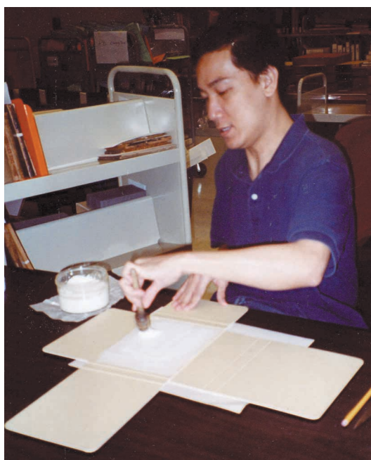
Figure 4. Applying adhesive to the center of the vertical board.
