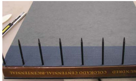
9. Comb pushed completely through textblock and covers
